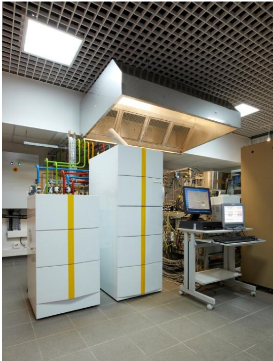
FC based mCHP system "Beta 0", co-developped by De Dietrich Thermique and CFCL, tested at GDF SUEZ CRIGEN fuel cell laboratory
